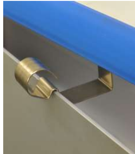
Figure 12 Details: Clip for keeping the doors open in the washing plant
