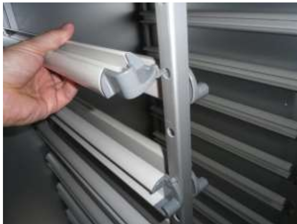
Figure 17 The assembly rails are suspended in the vertical bracket
