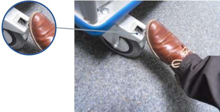
Figure 31 Releasing the wheel lock
